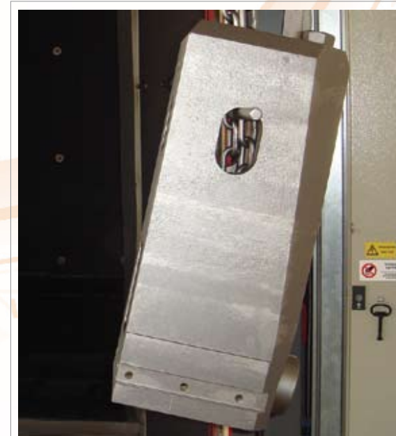
Sifone sabbiato Gooseneck after shot blasting
